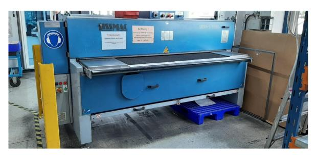
Deburring and edge rounding in one pass on both sides of steel and stainless steel sheet plate.
